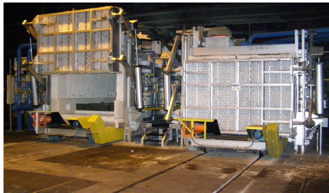
Twin 2,100° F Car Bottom Furnaces with Swing-Up style door and chain-driven furnace cars.
