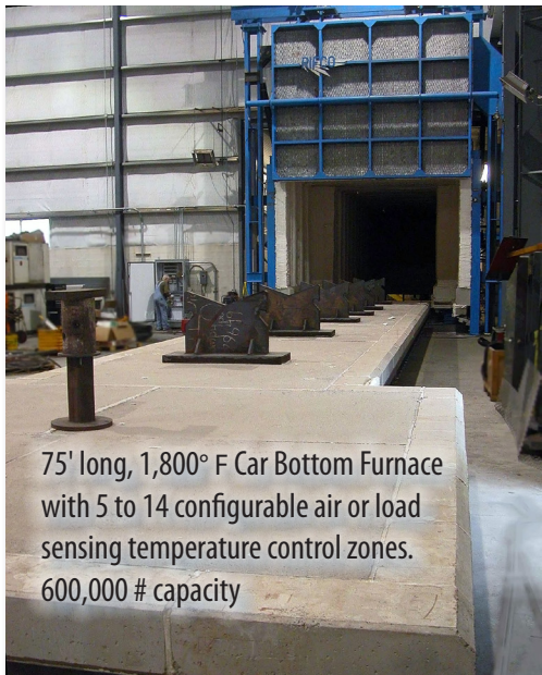
Car Bottom Furnace with Pulse-fired type combustion control system.
