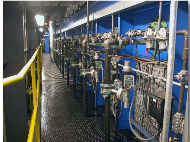
Car Bottom Furnace with Pulse-fired type combustion control system.
