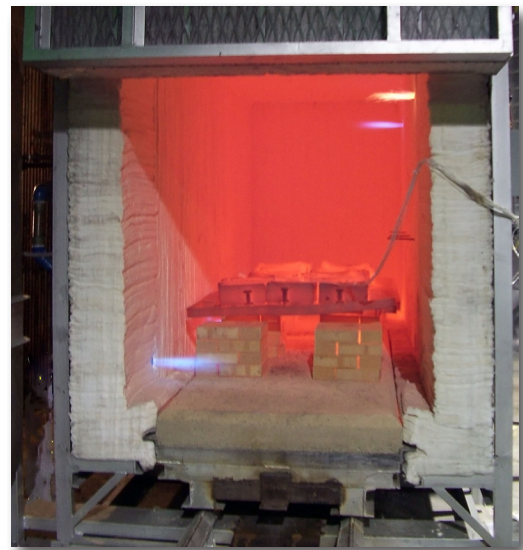
Pulse fired Car Bottom Furnace with manually driven furnace car.
