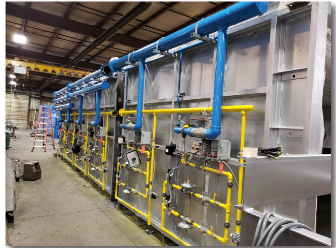
Modular design for a 3-zone, 40' deep High-Temperature (2,400° F) Industrial Box / Batch Furnace being staged for shipment.
