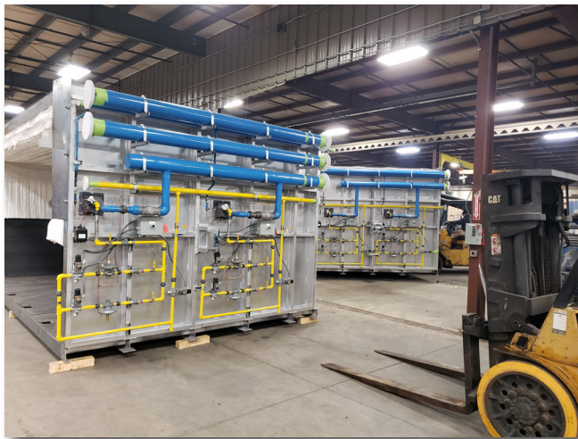
Modular design for a 3-zone, 40' deep High-Temperature (2,400° F) Industrial Box / Batch Furnace being staged for shipment.
