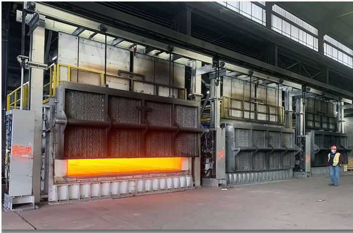
Turn-key project for three (3) High-Temperature (2,400° F) Industrial Box / Batch Furnaces designed and built for Carpenter Technology's #4 Hot Strip Mill in Reading, PA.
