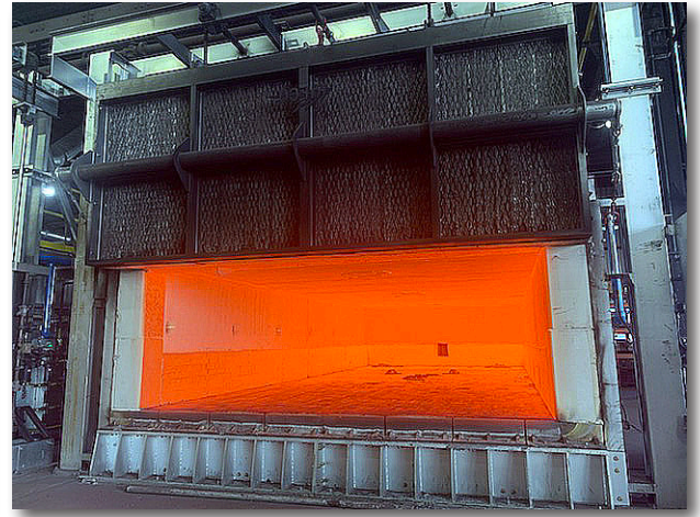
Turn-key project for three (3) High-Temperature (2,400° F) Industrial Box / Batch Furnaces designed and built for Carpenter Technology's #4 Hot Strip Mill in Reading, PA.
