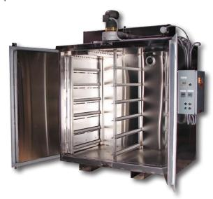
This oven was designed to remove moisture from refurbished electric transformers. It's large interior chamber accommodates a variety of load sizes.
