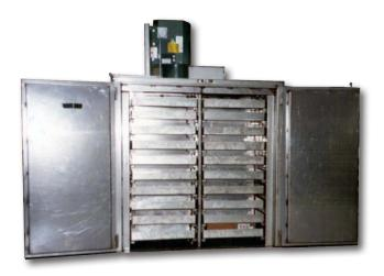
This steam heated curing oven was designed for the rubber industry.
