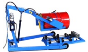
Load your drum onto Stationary Drum Rollers.
