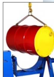
Place drum in holder with Drum Lifting Hook
