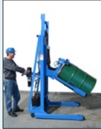
2. Tilt drum to horizontal and transport to racking location.
