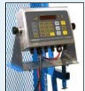
"N" Type scale indicator NOT for use in hazardous environments.
